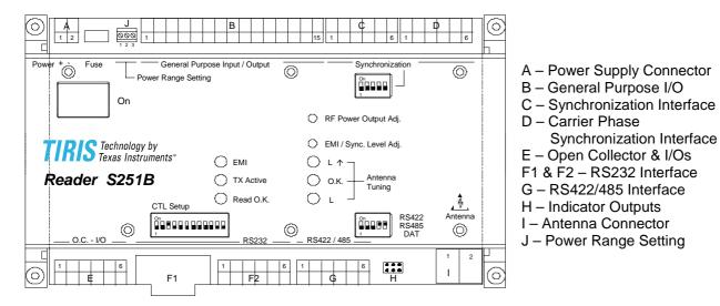
The default switch settings for "CTL Setup", "Synchronization" and "RS422/RS485/DAT" are shown in the figure above.
